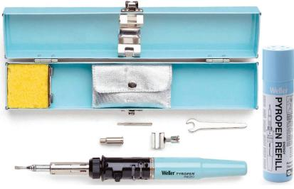
Powered by Butane gas, this Pyropen offers soldering iron, hot air blower and blow torch options. It has a short heat up time and can be refilled in seconds from a refill cylinder. A sight glass shows the level of gas in the reservoir. Temperature control is acheived by increasing and decreasing the gas flow.
